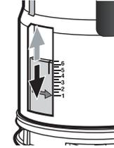
8. Adjust the full flush volume by sliding the red part up or down. when the buoy is higher. the discharge water volume is less. slide down the part can buoy little until you are flushing enough water.
