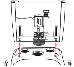
6. Fasten the tank to bowl with one pair of plastic or stainless steel bolts. Make sure bolts have the black rubber washer under the bolt's head.
