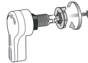
2. Unscrew the flanged nut from the handle body and remove the square seal.
