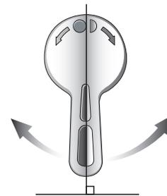
4. Make sure the handle in vertical position, it swings left and right approx. 90degrees
