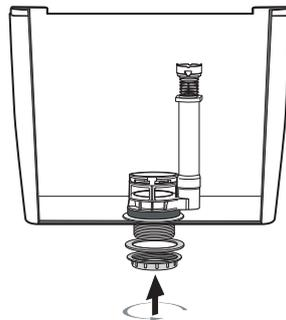
3. Insert the flush valve's base into the water tank. Screw on the nut collar and hex nut properly.
