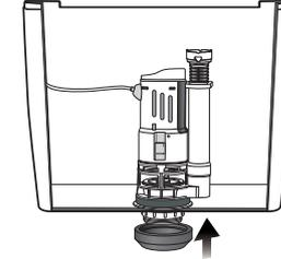
5. Insert the tank to bowl rubber gasket on to the flush valve's outlet bottom.
