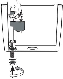
1. Insert the new fill valve with silicon seal at the base into the inlet hole of water tank and screw on the nut with collar tightly.
