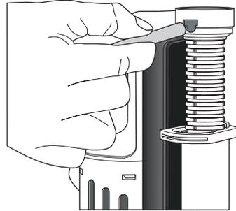
2. Connect the toilet bowl refilling tube from fill valve to the overflow pipe of flush valve.
