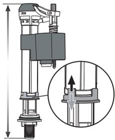
3. At the base of the fill valve's outer body unlock the fix stopper (see picture) by turning it counterclockwise then free up the inner body by pulling and or pushing on it.
