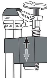
4. Fine and final adjustment can be made by rotating the screw rod clockwise or counterclockwise in the fill valve cup.
