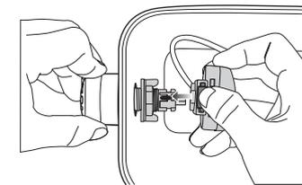
5. **Important!!!** Align the grooves on the handle mechanism in vertical position (see picture).
