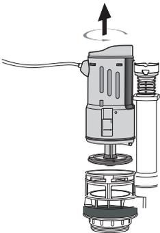
1. Hold the base of the flush valve and rotate the body counterclockwise take it out from base.
