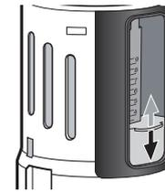
7. Adjust the half flush volume by sliding the marked part up or down. when the buoy is higher. the discharge water volume is less. slide down the part can buoy little until you are flushing enough water.
