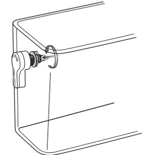
3. Insert the seal into the square hole on the water tank (fits only one way)
