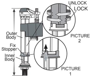
3. At the base of the fill valve's outer body, unlock the fix stopper (see picture 1) by pushing it down, then twist the outer body (see picture 2) clockwise to unlock. Adjust the outer body to the desired height. After setting it, twist the outer body counter clockwise to lock it to that position then pull the fix stopper upward to secure it.
