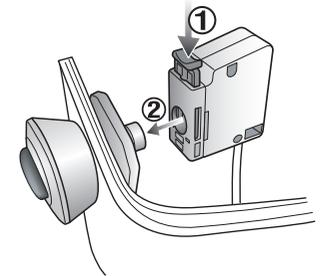
3. Push in switch box's green button (1) to connect with button body.
