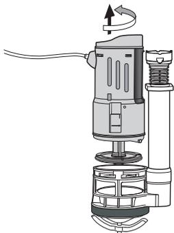
1. Hold the base of the flush valve and rotate the body counter-clockwise. Take it out from base.
