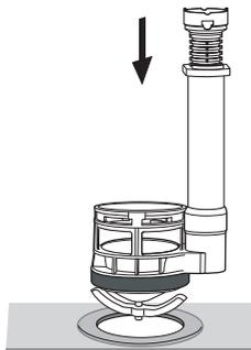
2. Put the base into the ceramic hole.
