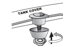
2. Insert the button into the oval hole of tank and then screw up cover and flanged nut in sequence.
