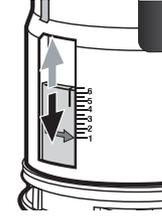
8. Adjust the full flush volume by sliding the red part up or down. When the buoy is higher, the discharge water volume is less. Slide down the buoy part until you reach the desired amount of discharged water.
