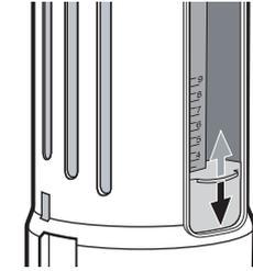
5. Adjust the half flush volume by sliding the marked part up or down. When the buoy is higher, the discharge water volume is less. Slide down the part a little until you are flushing enough water.
