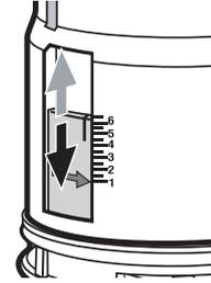
6. Adjust the full flush volume by sliding the red part up or down. When the buoy is higher, the discharge water volume is less. Slide down the part a little until you are flushing enough water.
