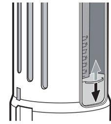
5. Adjust the half flush volume by sliding the marked part up or down. When the buoy is higher, the discharge water volume is less. Slide down the part can buoy little until you are flushing enough water.
