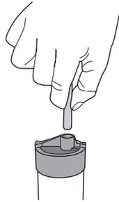
2. Connect the refill tube with refill restrictor from fill valve to the overflow pipe of the flush valve.
