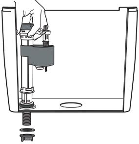
1. Insert the new fill valve with rubber seal at the base in the inlet hole of water tank and screw on the nut with collar tightly.
