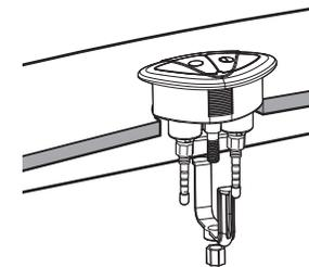
Insert Button Body in the button hole of lid and separately level the Full Flush Button and Partial Flush Button of Push Button at those of Flush Valve, then load U Buckle into Button Body (as picture) and screw Fix Nut to U Buckle tightly.
