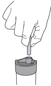
2. Connect the refill tube with refill restrictor from fill valve to the overflow pipe of the flush valve.
