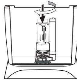
4. Take the body of flush valve and set it into the base and lock in place by rotating it clockwise.
