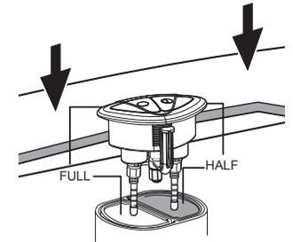
Loose Eight-square Nut and adjust the height of Rod to expected, then screw Eight-square Nut tightly.
