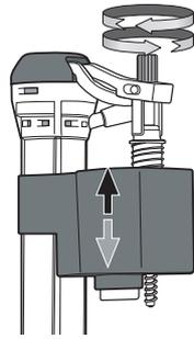
4. Fine and final adjustment can be made by rotating the screw rod clockwise or counter-clockwise on the fill valve cup. In order to achieve desired water level.
