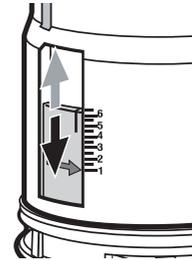
6. Adjust the full flush volume by sliding the red part up or down. When the buoy is higher, the discharge water volume is less. Slide down the part can buoy little until you are flushing enough water.
