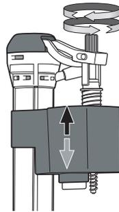
4. Fine and final adjustment can be made by rotating the screw rod clockwise or counter-clockwise on the fill valve cup. In order to achieve desired water level.
