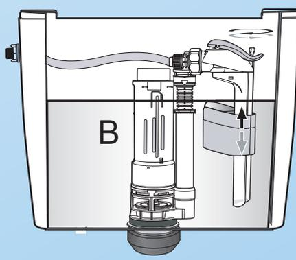
Connect the tube to the side of water tank.
