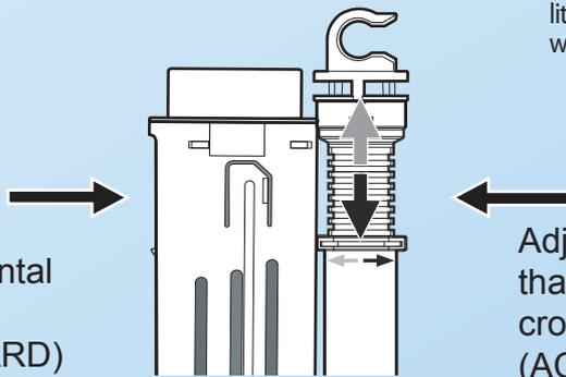
Adjust it to be 45mm higher than the water level when the horizontal cross-section is smaller than 300cm<sup>2</sup>. (ACCORDING TO ISRAEL STANDARD)
