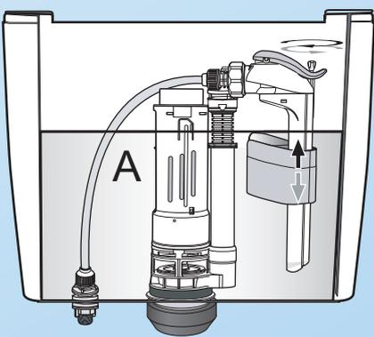
Connect the tube to the bottom of water tank.
