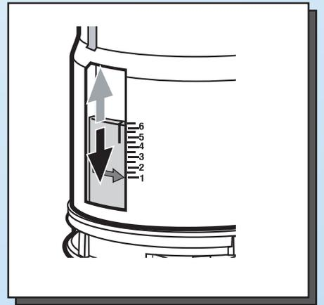
1b. Adjust the partial flush volume by sliding the green can buoy up or down. When the can buoy is higher, the discharge water volume is less at flushing. To set the right water volume for the partial flush to get the vortex in the bowl at flushing.
