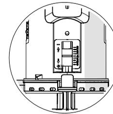
d. Micro HALF LOGO stand for the half flushing of fine-tuned window, it can adjust the half flushing of accurate water level when the half flushing of buoy at a minimum.
