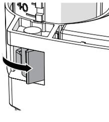
6. Rotate the buoy of lock buckle.
