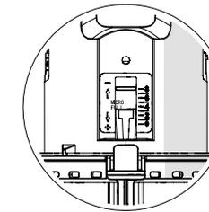
c. Micro FULL LOGO stand for the full flushing of fine-tuned window, it can adjust the full flushing of accurate water level when the full flushing of buoy at a minimum.
