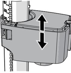
7. Pull the buoy up and down until adjust the suitable height.
