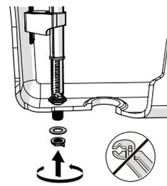
11. Install the fill valve into tank, rotate the gasket and nut.
