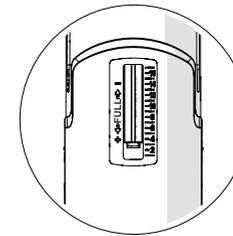
b. FULL LOGO stand for full flushing window, it can adjust the full flushing of water level more or less.
