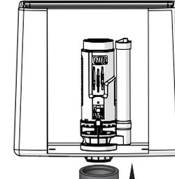
5. Install the rubber gasket at the bottom of the tank base.
