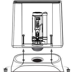
6. Take the water tank and install it on the two piece toilet of mounting holes, then fasten the bolts.
