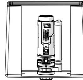
4. Take the body of the flush valve and install inside of tank. Put forth effort and push the body until two side of buckle lock the base.
