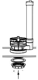
3. Insert the flush valve's base with rubber into the water tank, then screw on the plastic nut collar and hex nut properly.
