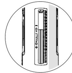
a. HALF LOGO stand for half flushing window, it can adjust the half flushing of water level more or less.
