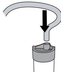
12. Insert the filling water hose of 10mm length into the overflow pipe inside.
